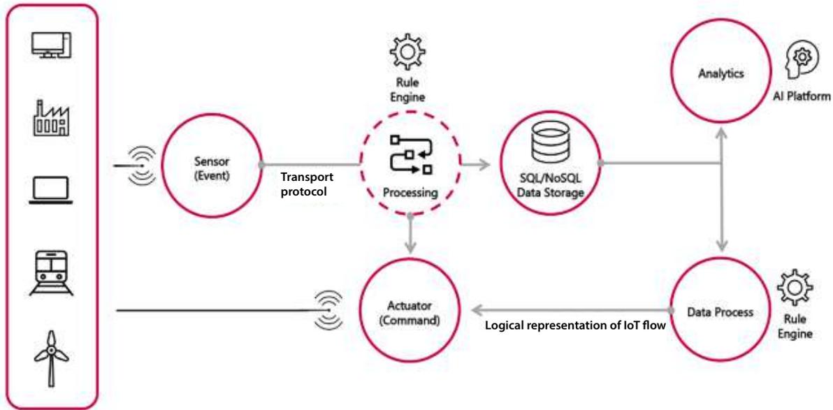
Starting from the macro-classification between **passive devices (sensors) and active devices (actuators)**, a sensor recognises certain environmental conditions of the context for which it was designed, encodes this information and transfers it via the Internet to a collection point for analysis.
